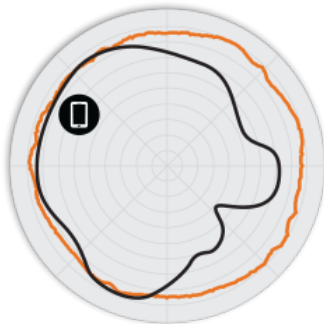
Figure 2. R310 2.4GHz Azimuth Antenna Patterns
